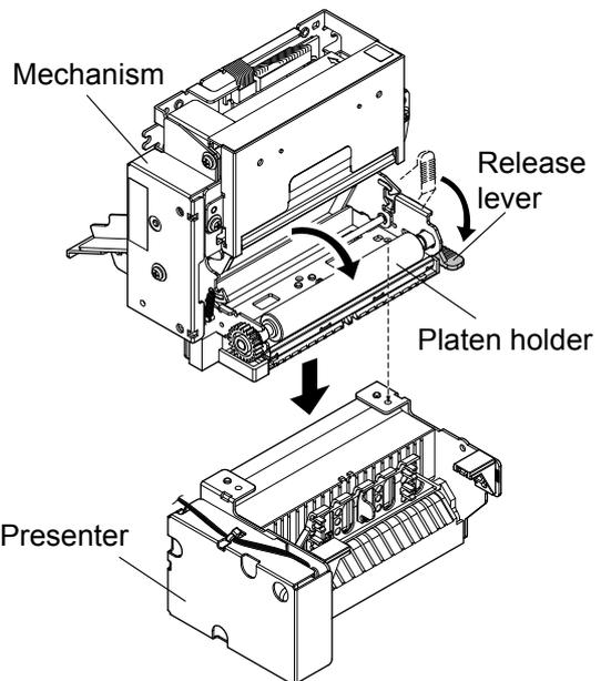
2. Position the screw holes as shown on the right, and place the mechanism on top of the presenter.
