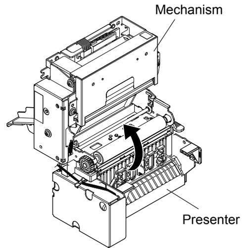
5. Using the two M3x5 screws, attach the ground wire to the mechanism and the presenter.
