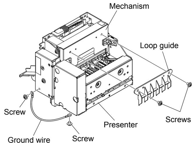
7. Place the mechanism so that the paper outlet faces up (see the diagram on the right).
